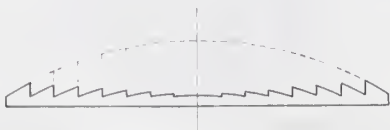
Cross section of a Fresnel lens indicating its construction
